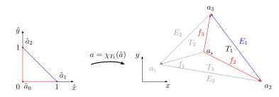
Figure 2: Mapping between the reference triangle and  $T_1$
