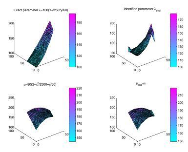
Figure 3: Identification of parameter  $\lambda$  with Tikhonov regularization, identification error  $\approx 11.6\%$
