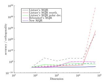
Figure 4: Accuracy and orthogonality (dotted) for the BEM example series
