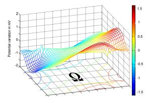
Figure 3: Variation of the potential field in mV for  $\varepsilon_x=0,\ \varepsilon_y=0,\ \gamma=0.005$  compared with the potential for undeformed state  $\varepsilon_x=\varepsilon_y=\gamma=0$  (supply voltage of  $U_B=2V$ )
