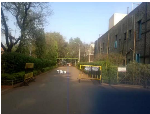
Figure 3.1: Depth Estimation using the Vertical Position of the Bounding Rectangle. The yellow Line is located at the Vertical Position of the Vanishing Point [23].
