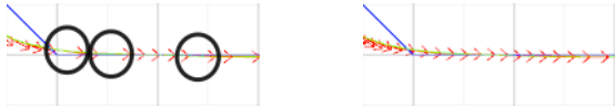
Fig. 7. Comparing the spacing of adjacent poses. Left: due to the internal logic of the TEB-planner, the poses have sometimes greater spacing. Right: our implementation solve the inequality. This was necessary to allow easier visual comparison between different generated trajectories.
