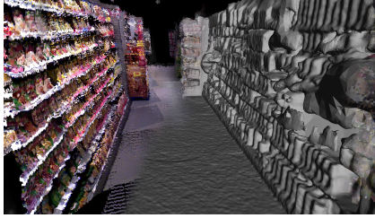
Fig. 2. The result of the supermarket pointcloud and its resulting mesh (left to right is going from points to surface).
