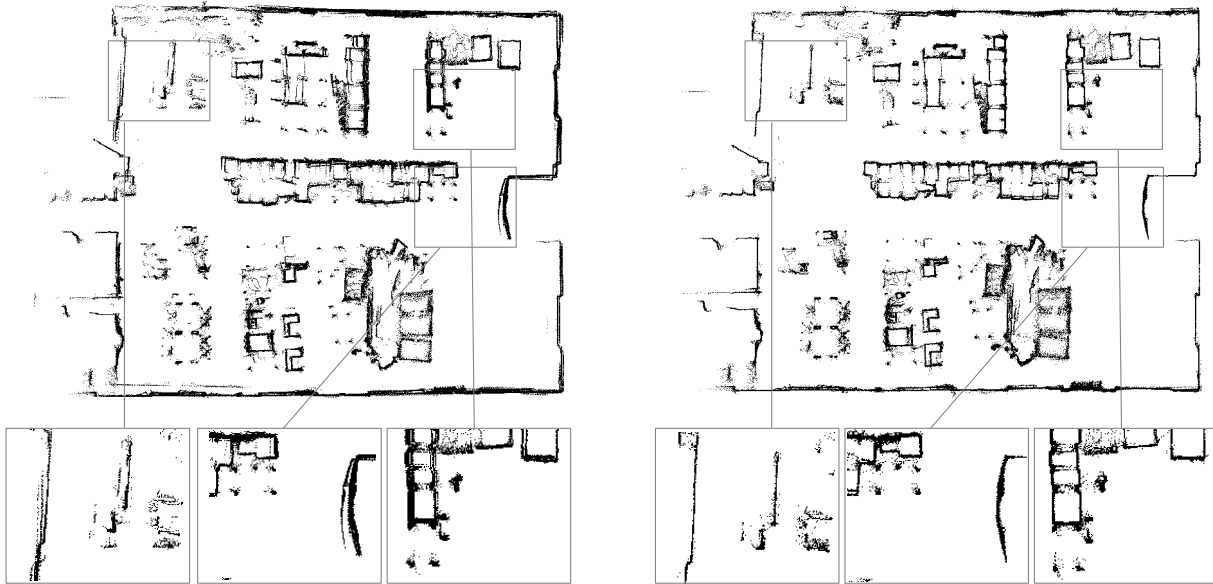
(a) Initial input obtained from pose graph SLAM. Some walls appear twice in the map. Fine local structures are not accurately captured and seem spread around objects.
