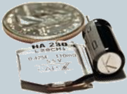
Mini-Supercap von Cap-XX (0,425F @ 5,5V)
